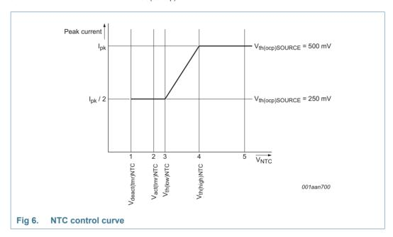
When the voltage on the NTC pin exceeds  $V_{th(high)NTC}$  (see <u>Figure 6</u> (4)), the converter delivers nominal output current. When the voltage is lower than this level, the peak current is gradually reduced until  $V_{th(low)NTC}$  is reached (see <u>Figure 6</u> (3)). The peak current is now half the peak current of nominal operation. When  $V_{act(tmr)NTC}$  is passed (see <u>Figure 6</u> (2)) a timer starts to run to distinguish between the following situations:
