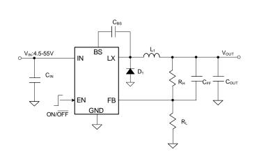
Figure 1. Typical Application Circuit
