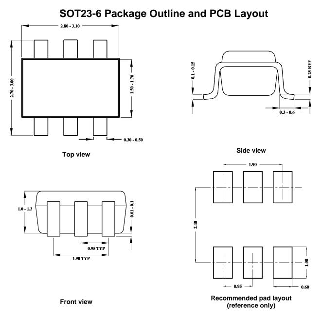
Note: All dimensions are in millimeters and exclude mold flash and metal burr.
