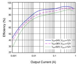
Figure 2. Efficiency vs. Output Current
