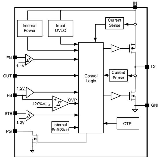
Figure 3. Block Diagram
