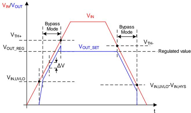
Figure 5. Bypass Mode Transition
