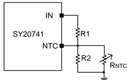
Figure 5. Alternate UTP /OTP configuration
