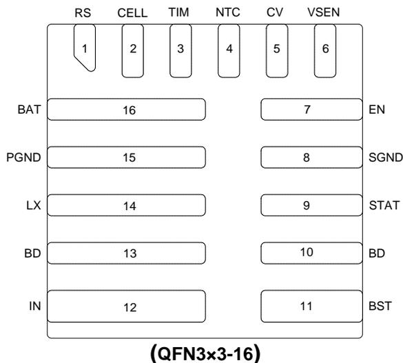
Figure 2 Package Pinout
