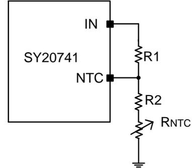
Figure 4. UTP /OTP configuration using  $R_1$  and  $R_2$
