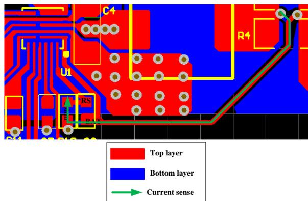
Figure 3. PCB Layout Suggestion
