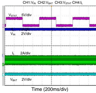
Steady Waveform When No Battery
