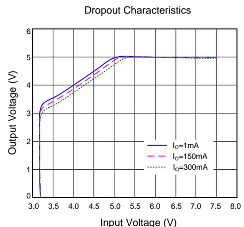
Figure 2. Dropout characteristics
