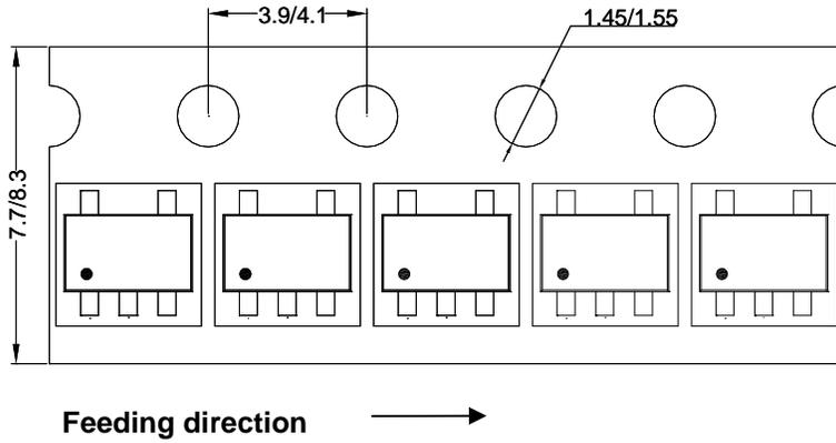
**Carrier tape and reel specification for packages**
