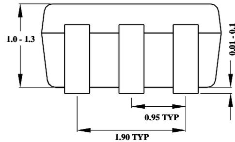
**Note:** All dimensions are in millimeters and exclude mold flash and metal burr.
