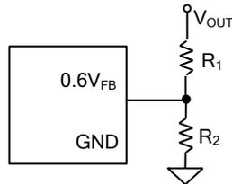
With a calculated value of 22.2kΩ for R2, a standard 1% 22.1kΩ resistor is selected.
