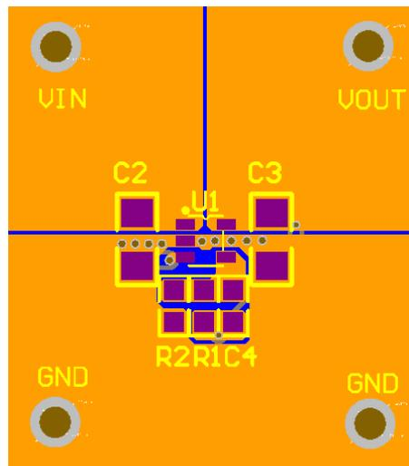
Figure 4. Recommended PCB layout
