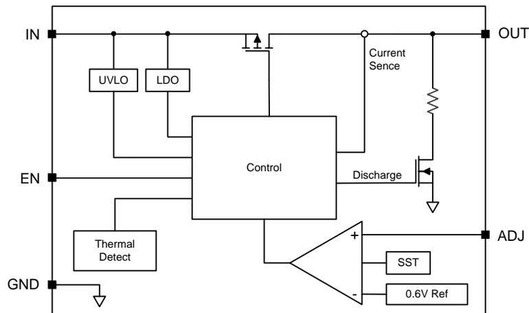
Figure 3. Block diagram
