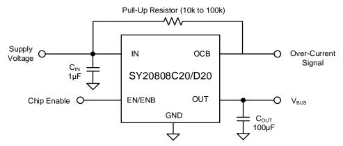
Note: If  $1\mu F$  input cap will lead to large Vin voltage spike, it is strongly recommended to add additional  $10\mu F$  ceramic cap.
