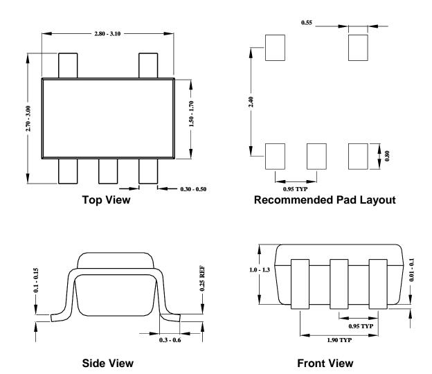
Note: All dimensions are in millimeters and exclude mold flash and metal burr.
