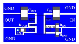
Figure 2. PCB Layout Suggestion
