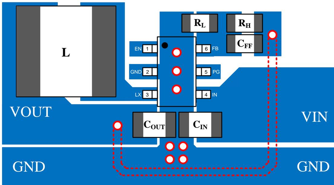
Figure 4. Recommended PCB Layout
