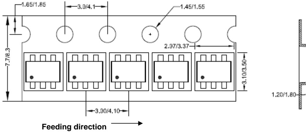
**Carrier tape and reel specification for packages**
