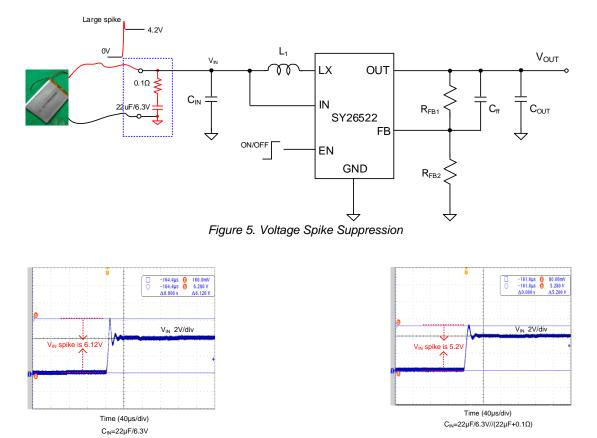
Figure 6. Voltage Spike without Suppression
