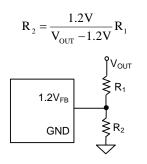
Figure 4. Feedback Resistor Divider
