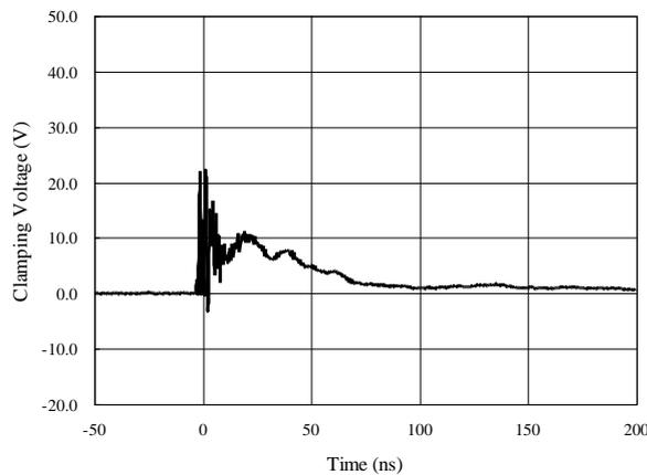
**ESD Clamping of I/O to GND
