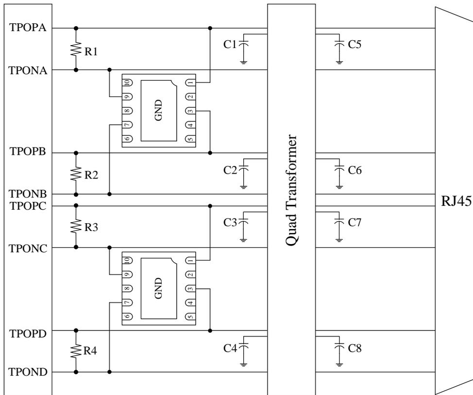
Schematic Diagram for Gigabit Ethernet ESD/Surge Protection using SYS11L03SEC
