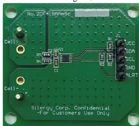
Figure 3 SY6410 Demo Board Top View
